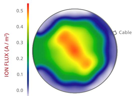
Figure 1: Spatial distribution of the ion flux to an RF biased substrate measured with the Semion™ Multi Sensor
