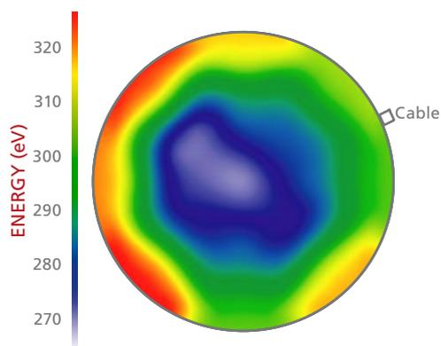
**Figure 2:** Spatial distribution of the average ion energy to an RF biased substrate measured with the Semion™ Multi Sensor
