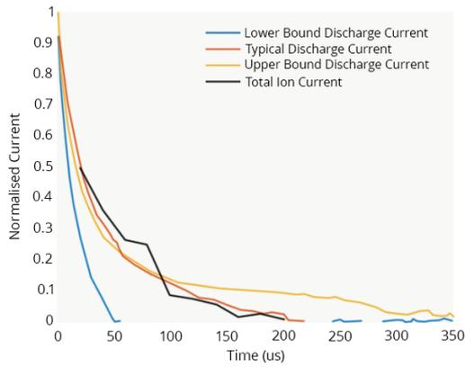
Figure 2. Temporal evolution of the Normalised discharge current and total ion current.
