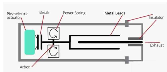
Figure 1. Schematic diagram of the ISF-VAT.
