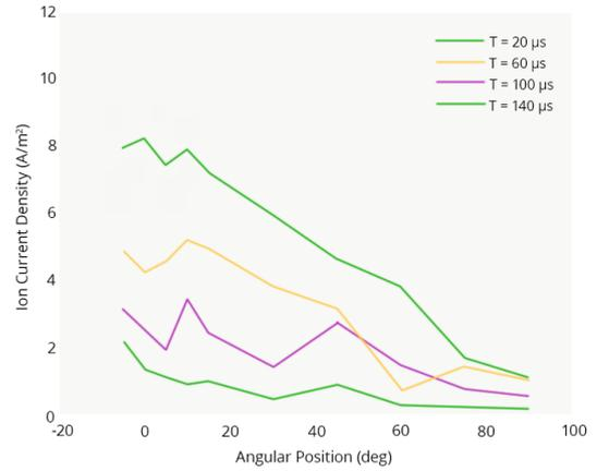
Figure 3. Ion-current density as a function of the azimuthal angle where  $0^\circ$  represents the direction the thruster is pointed.
