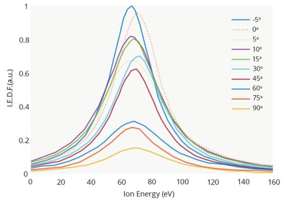
Figure 4. IEDF for different azimuthal positions ranging from  $-5^\circ$  to  $90^\circ$ .
