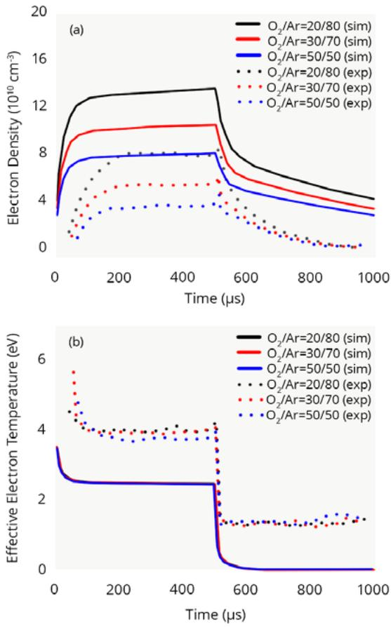
Figure 2. Temporal evolution of the electron density and effective electron temperature for various Ar/O<sub>2</sub> plasmas.
