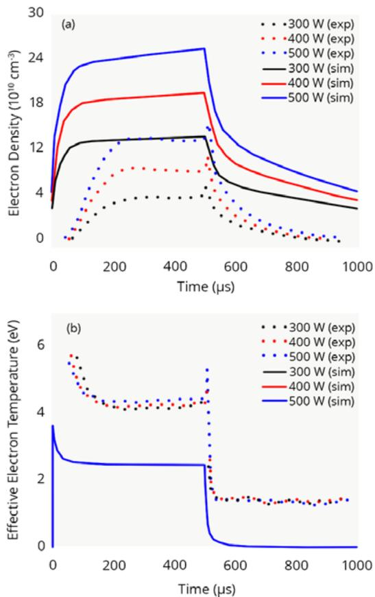
Figure 4. Temporal evolution of the electron density and effective temperature for various powers.
