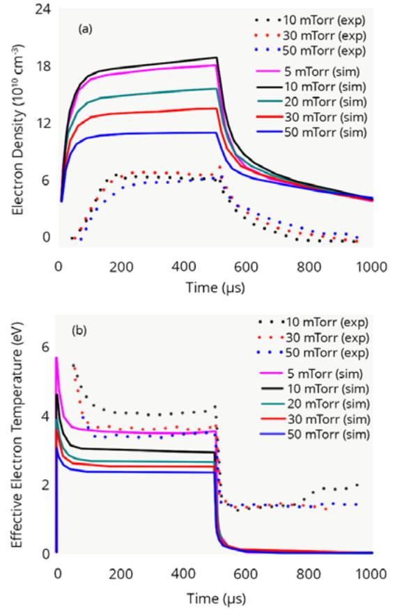
Figure 3. Temporal evolution of the electron density and effective electron temperature for various pressures.
