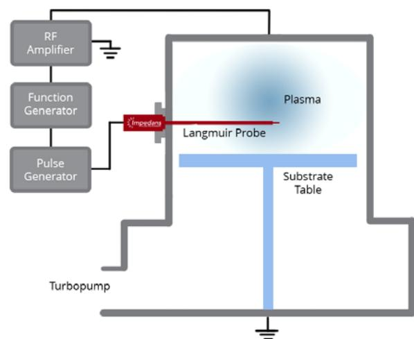
Figure 1. Schematic diagram of the Inductively Coupled Plasma Reactor.
