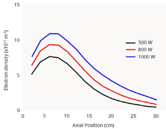
Figure 2. Axial spatial evolution of the electron density at a fixed pressure of 1 Pa for powers ranging from 500- $\rightarrow$ 1000 W.
