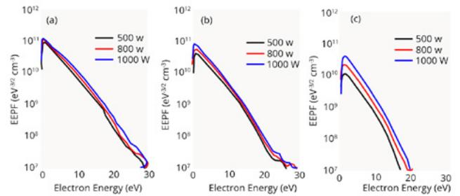
Figure 4. The EEPF vs applied power at the axial positions of (a) 6 cm, (b) 14 cm and (c) 24 cm at 1 Pa.
