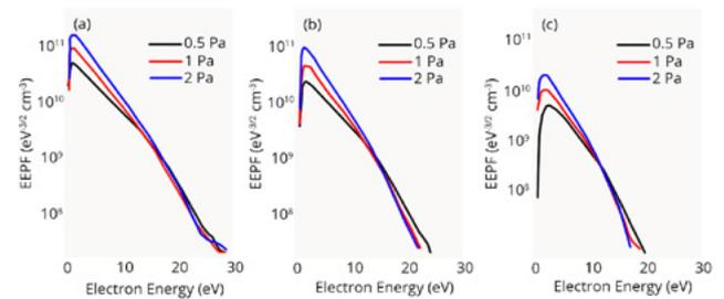
Figure 5. The EEPFs vs pressure at the axial positions of (a) 6 cm, (b) 14 cm and (c) 24 cm at 500 W.
