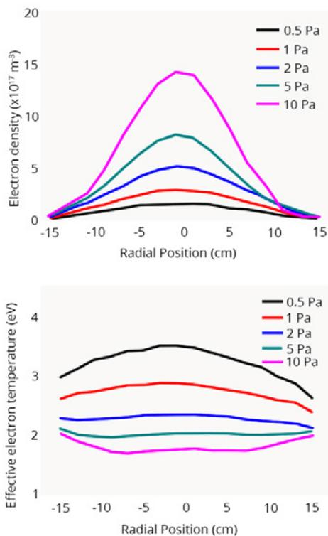
Figure 4. Radial distribution of the electron (a) density and (b) effective temperature for various pressures at 800 W.
