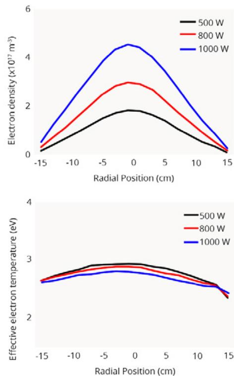
Figure 6. Radial distribution of the electron (a) density and (b) effective temperature for various powers at 1 Pa.
