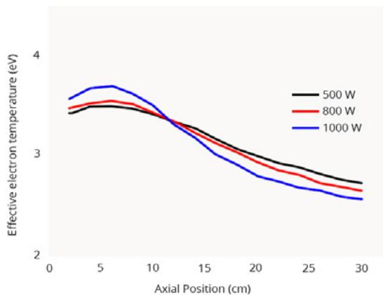
Figure 3. Axial spatial evolution of the effective electron temperature at a fixed pressure of 1 Pa for powers ranging from 500- $\rightarrow$ 1000 W.
