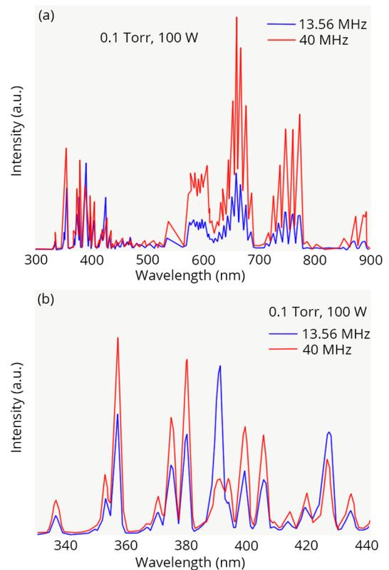
Figure 5. Two frequencies 13.56 MHz and 40 MHz for the whole spectrum (a) and zoomed spectrum (b).
