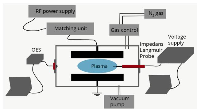
Figure 1. Schematic of the cyclic ALE process.
