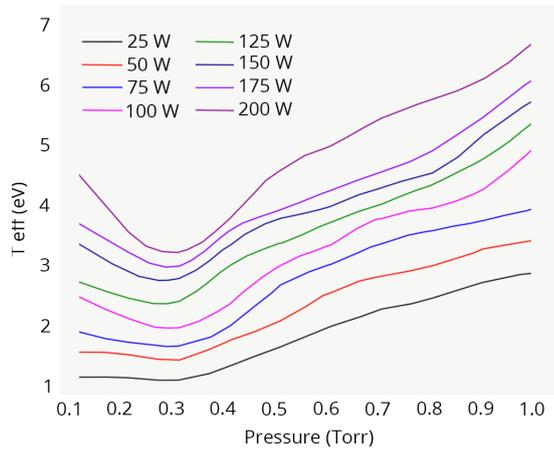
Figure 4. Effective electron temperature ( $T_{eff}$ ) is shown for 13.56 MHz.
