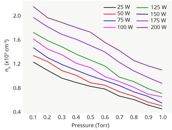
Figure 3. Electron density  $n_e$  is shown for 13.56 MHz.
