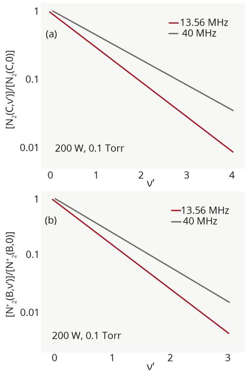
Figure 6. Boltzmann plots for  $N_2(C, v')$  vibrational distribution (a) and  $N_2^+(C, v')$  vibrational distribution (b) at 200W and 0.1 Torr for frequencies 13.56 MHz and 40 MHz.
