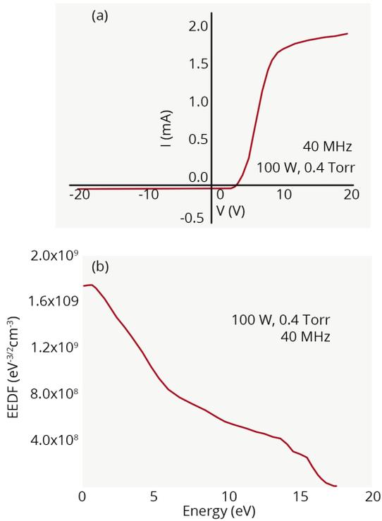
Figure 2. I-V curve (a) and EEDF (b) are shown for 40 MHz frequency.
