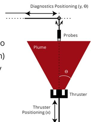
**Figure 1:** Schematic view of the HET and probe positioning system
