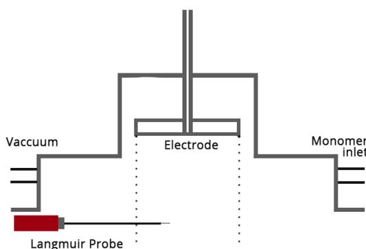
Figure 2. Top view of Langmuir probe setup within the plasma chamber.
