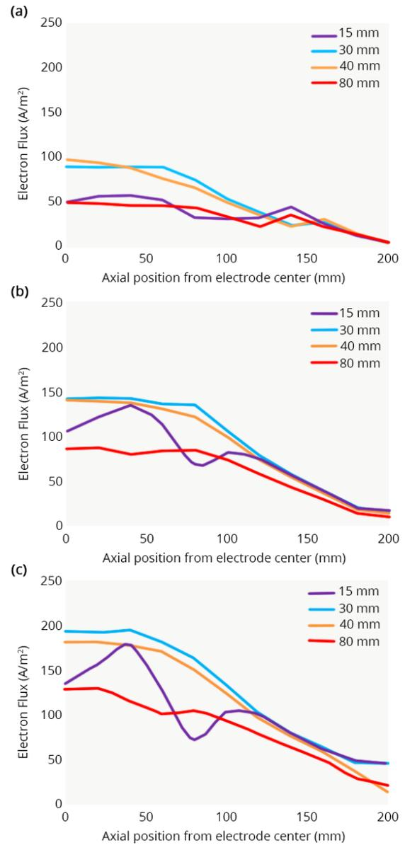
Figure 3. Electron flux measured using the Langmuir probe for RF powers of (a) 5 W, (b) 20 W and (c) 50 W at distances of 15, 30, 40 and 80 mm from the electrode.
