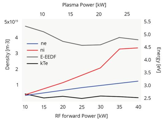
Figure 4. Temporal evolution of the electron density and effective temperature for various powers.
