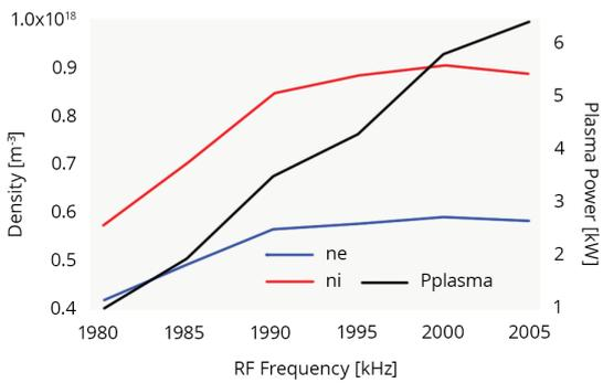
Figure 2. The dependence of  $n_e$ ,  $n_i$  and the plasma power on the RF frequency when applying a forward power of 10 kW.
