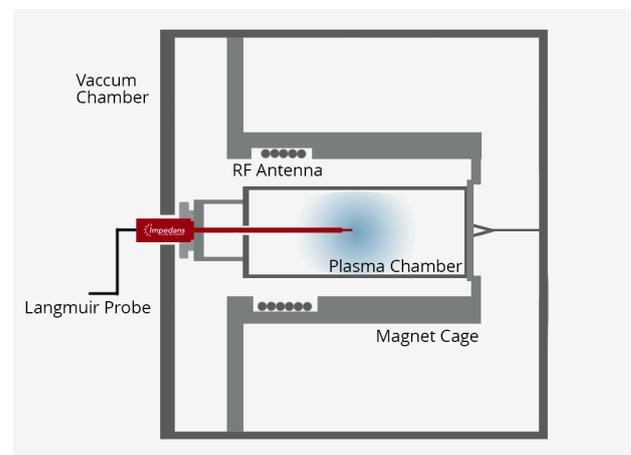
Figure 1. Schematic of the SPL plasma generator.
